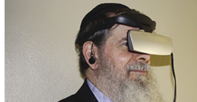
Thirty years after the release of his Accommotrac Vision Trainer, Joseph Trachtman, pictured here, released a home version of the device, called the Zone-Trac. Advances in technology made it possible for Trachtman to build a much smaller, wearable, and more affordable device.
